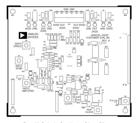
Figure 25. Evaluation Board Layout, Primary Silkscreen
