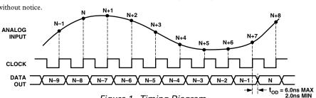
Figure 1. Timing Diagram
