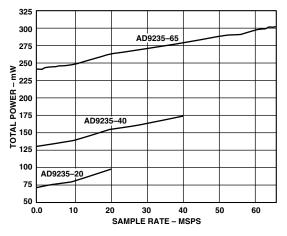
Figure 11. Total Power vs. Sample Rate with  $f_{IN} = 10 \text{ MHz}$
