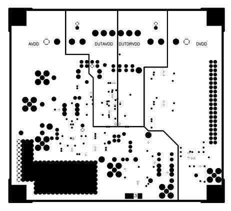
Figure 24. Evaluation Board Power Plane
