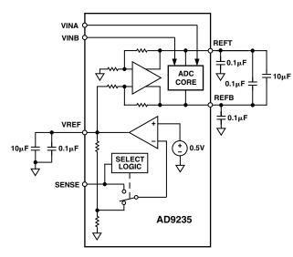
Figure 12. Internal Reference Configuration
