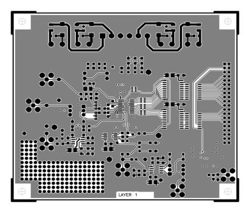
Figure 21. Evaluation Board Layout, Primary Side
