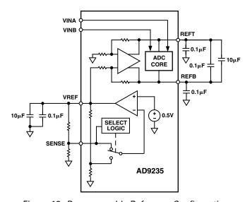
Figure 13. Programmable Reference Configuration
