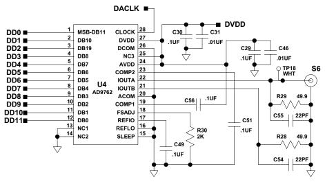
Figure 20. Evaluation Board Schematic, Optional D/A Converter
