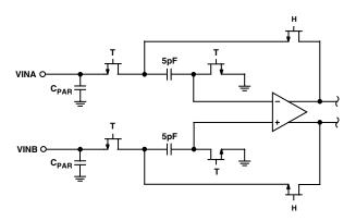
Figure 6. Switched-Capacitor SHA Input
