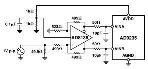
Figure 8. Differential Input Configuration Using the AD8138
