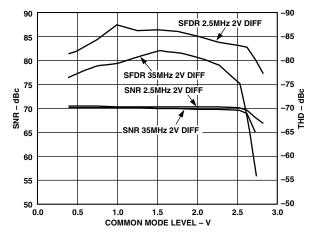
Figure 7. AD9235-65: SNR, THD vs. Common-Mode Level
