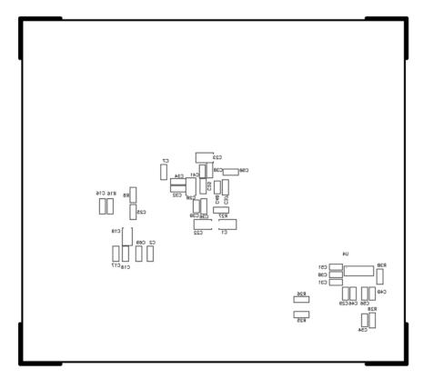
Figure 26. Evaluation Board Layout, Secondary Silkscreen
