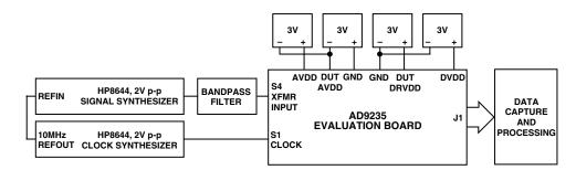
Figure 16. Evaluation Board Connections
