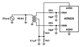
Figure 9. Differential Transformer-Coupled Configuration
