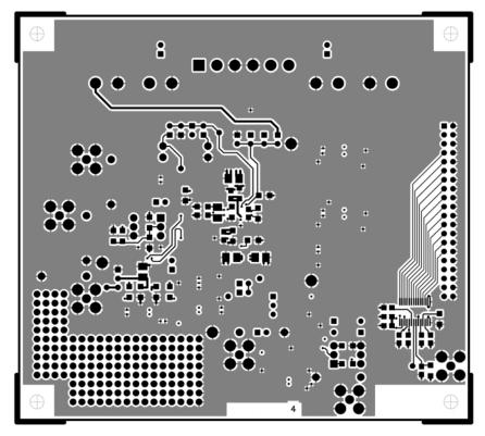
Figure 22. Evaluation Board Layout, Secondary Side
